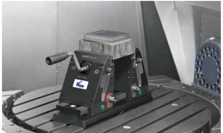
Pull-down clamping with the KIPPflexX centric vice function. Both jaws are locked, so that when force is applied - by deflecting the clamping jaws - a pull-down effect is produced towards the workpiece support.
