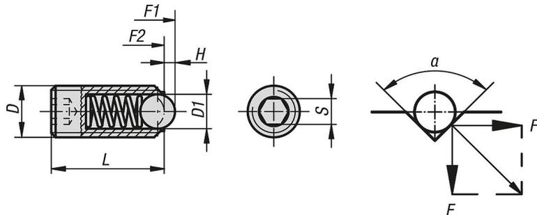
$$\begin{aligned} \alpha = 60^\circ, F' &= 1,732 \times F \\ \alpha = 90^\circ, F' &= F \\ \alpha = 120^\circ, F' &= 0,577 \times F \end{aligned}$$
