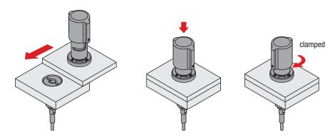
Check that the twist knob is in the "OFF" position and that the pin is retracted. Place the ball lock pin over the receiving bush or insert it. Press the twist knob down and turn it to the "ON" position. When fully clamped, an audible click will be heard.
